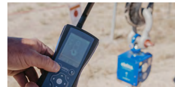
This remote raises and lowers the hook, allowing LLW to be placed in a trench and the hook to be removed without manual effort by operators.
