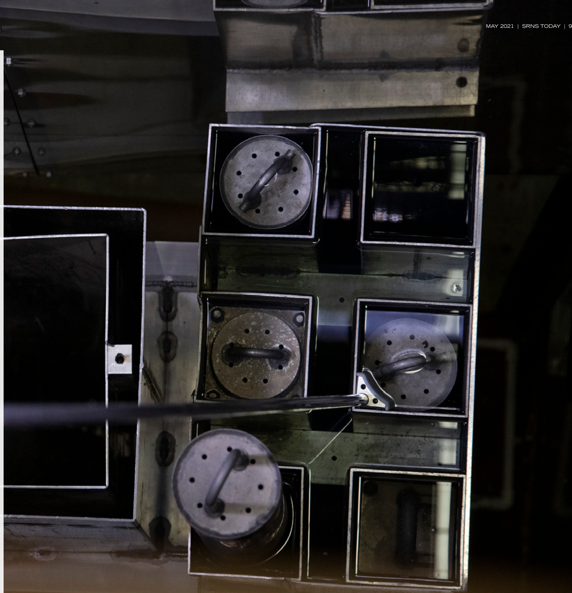
The camera in position over the fuel bundle to be inspected in the mockup
