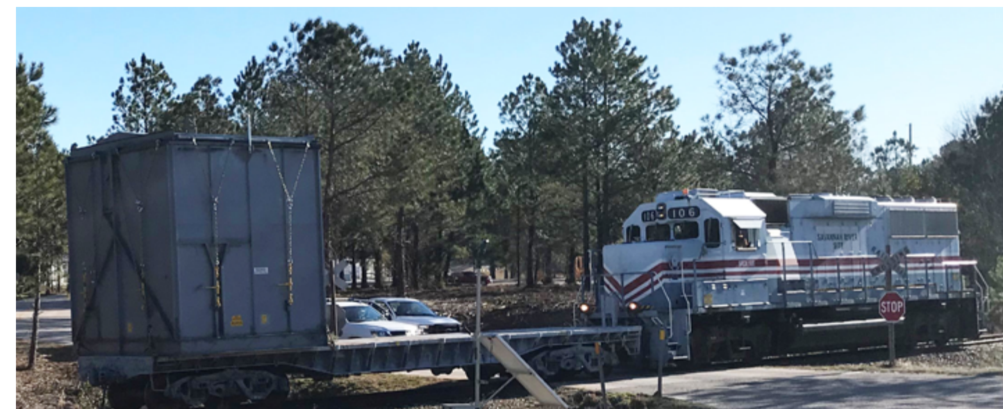
A train engine pushes a burial box full of failed equipment from H Canyon to the Solid Waste Management Facility for disposal. The equipment is being removed to make way for a new H Canyon spent nuclear fuel dissolving campaign.
