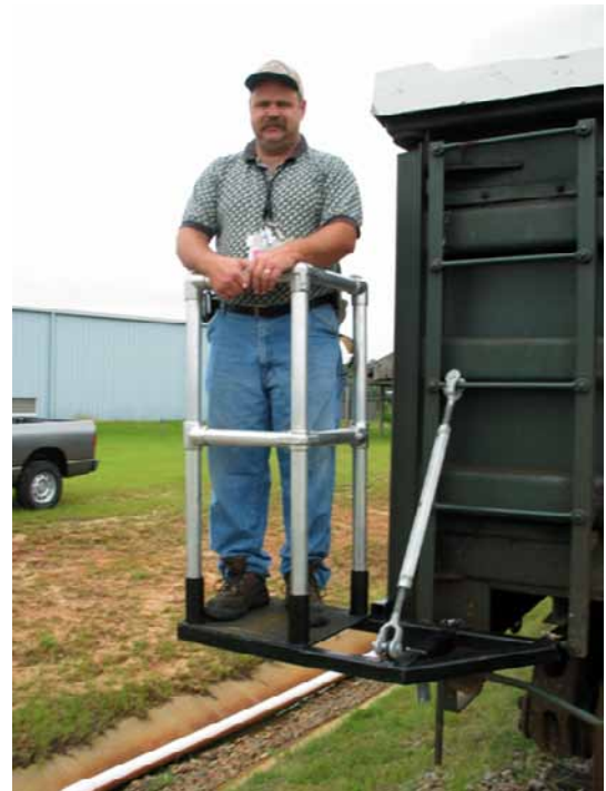
The platform can be used by railcar switchmen for enhanced safety and is rated for 300 pounds, load tested at 450 pounds.
