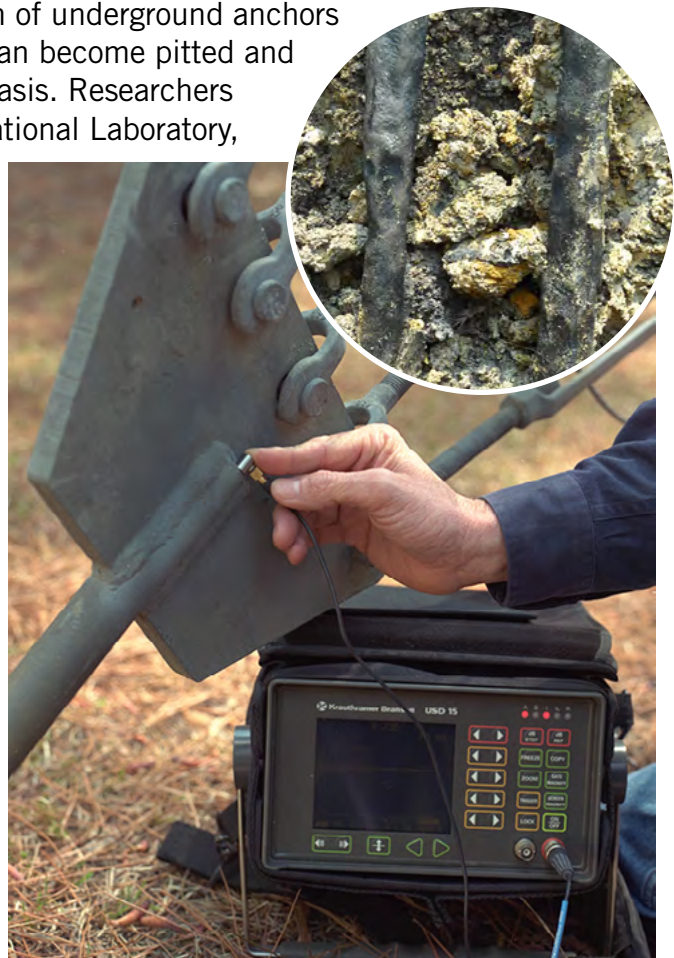
SoundAnchor™ device testing integrity of anchor rods (inset: Corroded anchor rod at test location)
