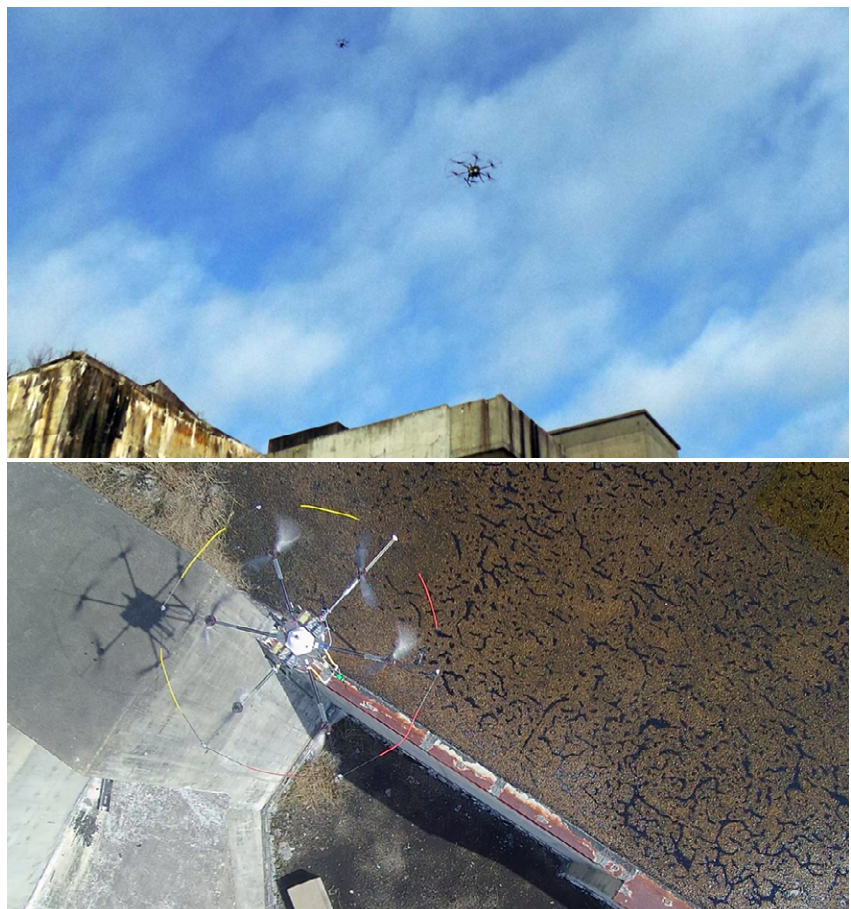
A small aerial drone (top) with a high-resolution camera hovers above a larger drone (bottom) that identifies where to spray herbicide on the rooftop of a closed reactor building at the Savannah River Site.
