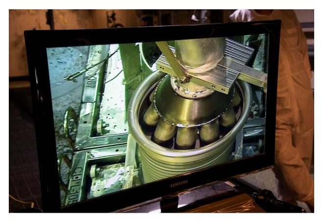
A team of SRS employees designed and installed a High Flux Isotope Reactor core cleaning station and vacuum tooling to ensure continued processing of spent nuclear fuel stored in the Site's L Basin.
