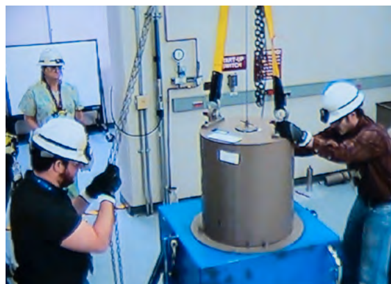
Replacing the source in the irradiator
