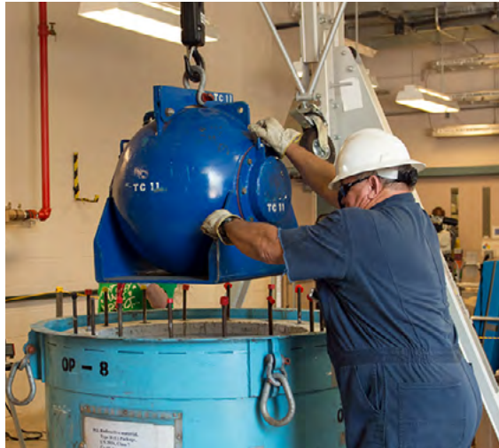
Removing the protective cask carrying a cobalt-60 source
