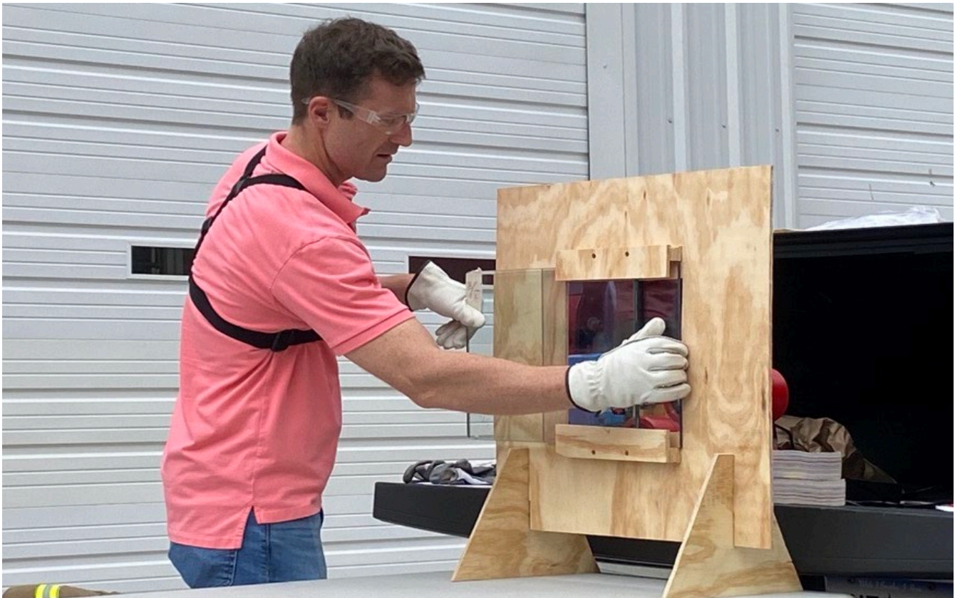
Andrew Kricke, SRNS Associate Fire Protection Engineer, tests various types of glass and their impact on the accuracy of flame detectors during his University of South Carolina Aiken Capstone project.
