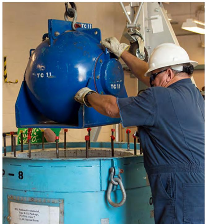
SRNS Employees remove the shielded cask carrying a Cobalt 60 source, used for the calibration of radioactivity monitors at SRS.
