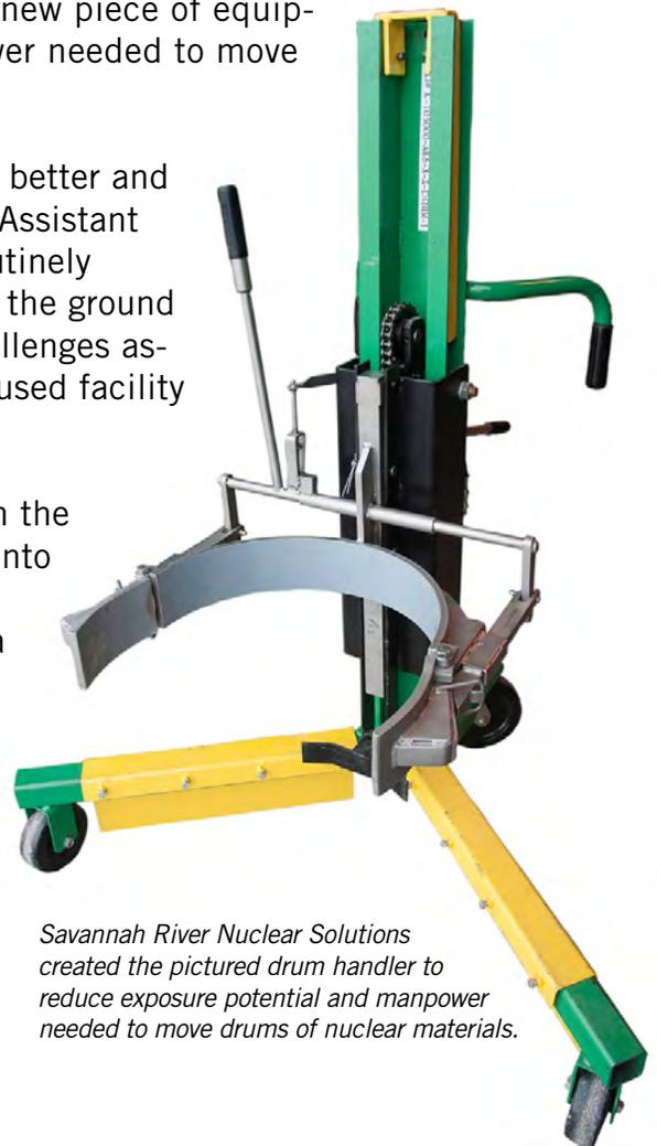
*Savannah River Nuclear Solutions created the pictured drum handler to reduce exposure potential and manpower needed to move drums of nuclear materials.*
