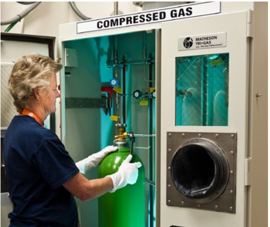
Operator Cindy Sizemore installs a tank to be filled with helium-3, a byproduct of the tritium manufacturing process.
