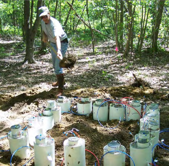
Science Fellow Charles Turick leads a field experiment to feed bacteria in an effort to stabilize potential soil contamination.
