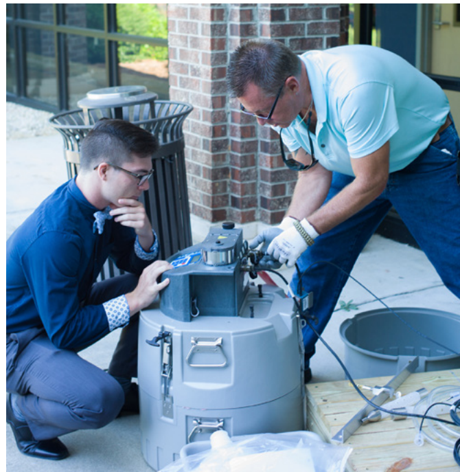
Caleb DiPrete (left) and Yaz Yascavage (right) set up the portable sampler that collects water quality data.
