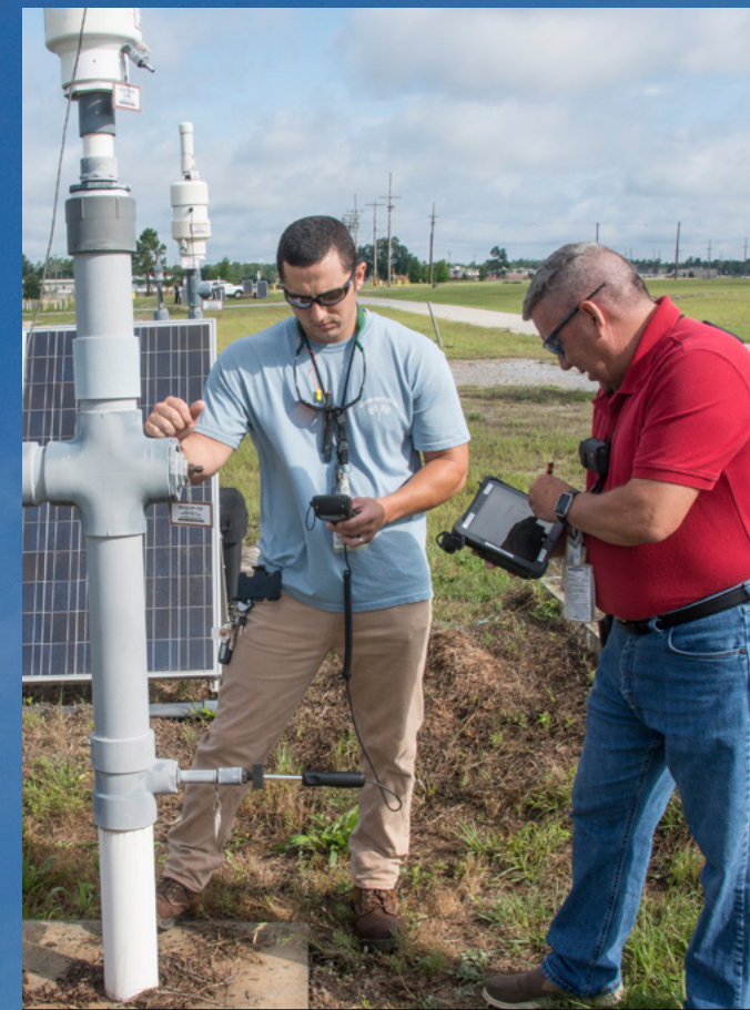
Remote Operators Matthew Easley (left) and Tony Craps take readings at one of 87 MicroBlowers used to passively remove chemical solvents at SRS.
