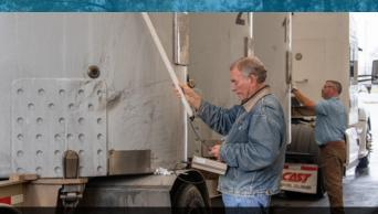
Shipping containers are surveyed to ensure no radiation is present before leaving SRS.
